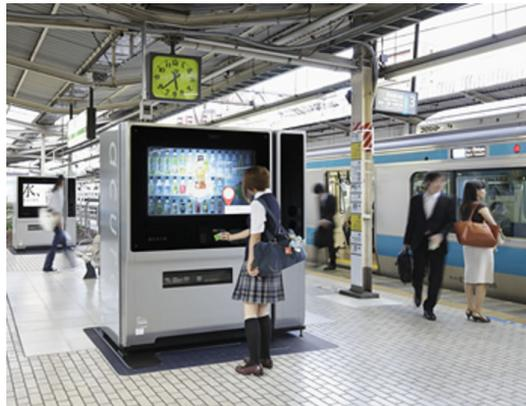
The figure shows a vending machine used for the experiment on a train platform. There is a digital touch panel in the front and a camera at the top of the machine recognizes the customer's age and gender. The vending machine makes recommendations based on the observed consumer characteristics. The image is supplied by the company.
